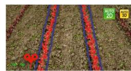
CULTI CAM was developed for automatically steering cultivators in row crops. The system detects the rows and guides the hoe along the crop with inchperfect precision. As well as 2D colour segmentation, the system also features a stereo camera for 3D object detection.
